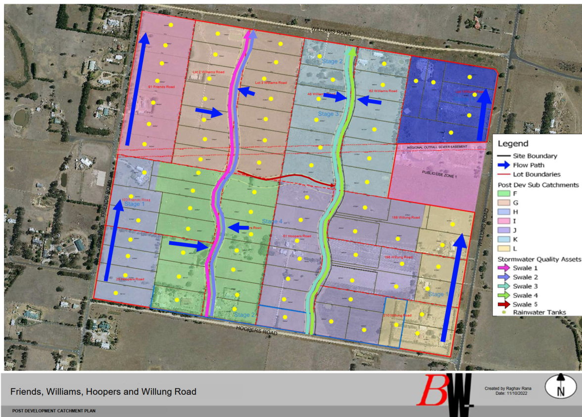
Figure 8: Stormwater Quality Assets
