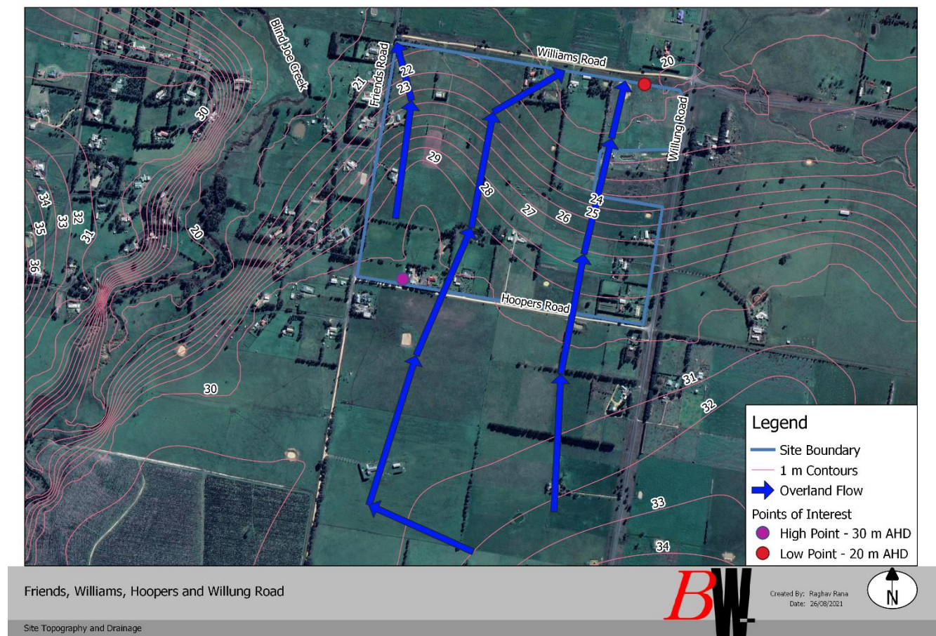
Figure 2: Surface Water Flow Direction
