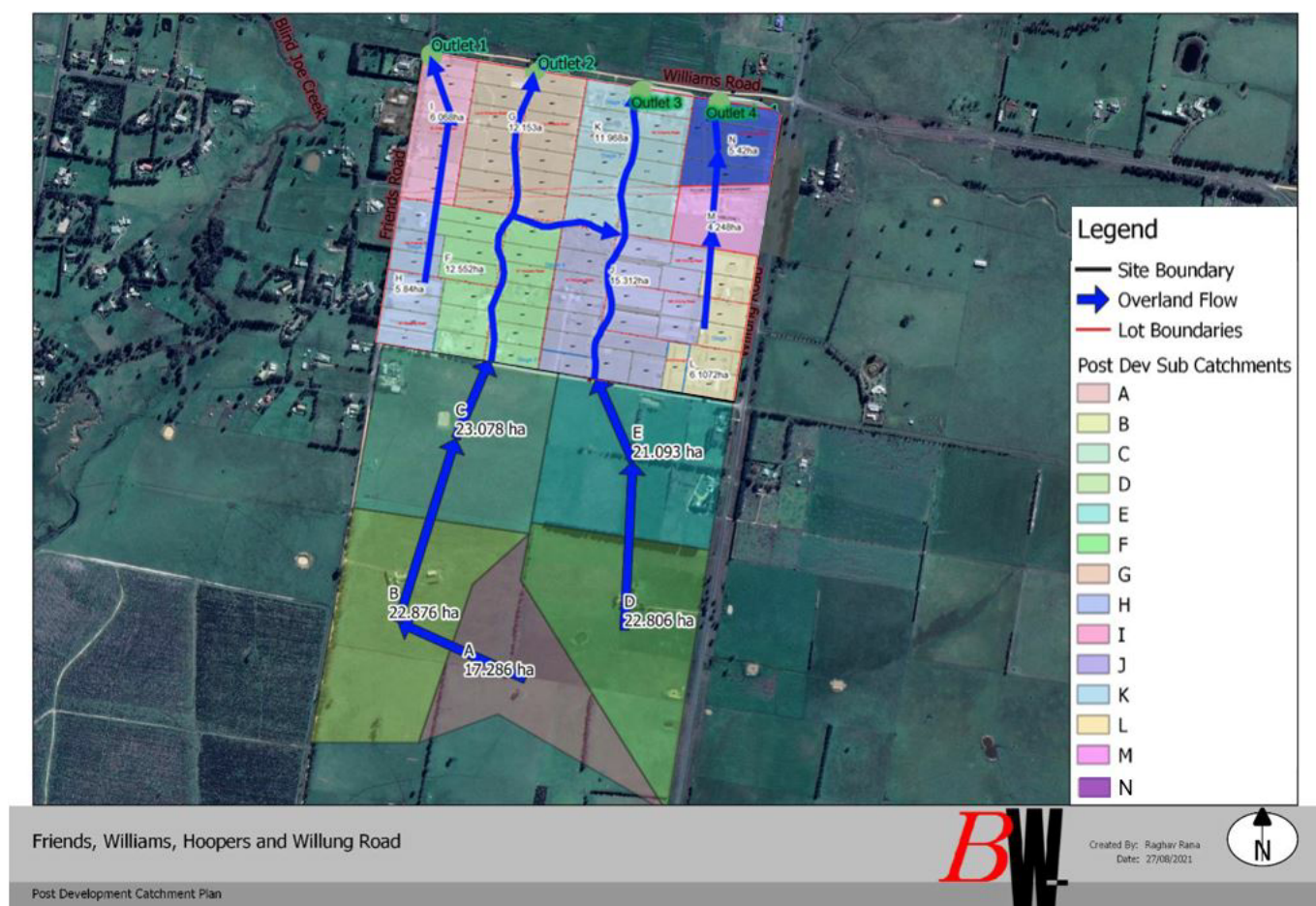
Figure 5: Post-Developed Catchment Plan (Not to scale)
