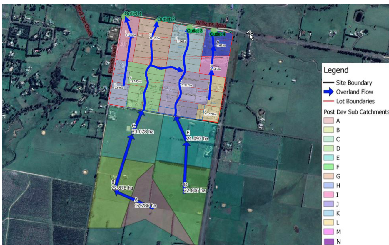
Figure 6: Site Overland Flow Path
